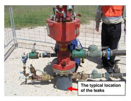
Photo of a typical well head – majority of the detected gas readings were recorded at the threaded connection between the steel casing pipe and the well head base at ground level (see red arrow).
